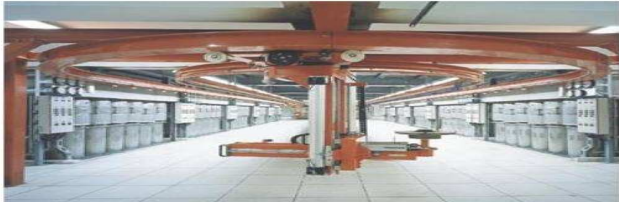
Staple fiber spinning lines with spin pack handling system
